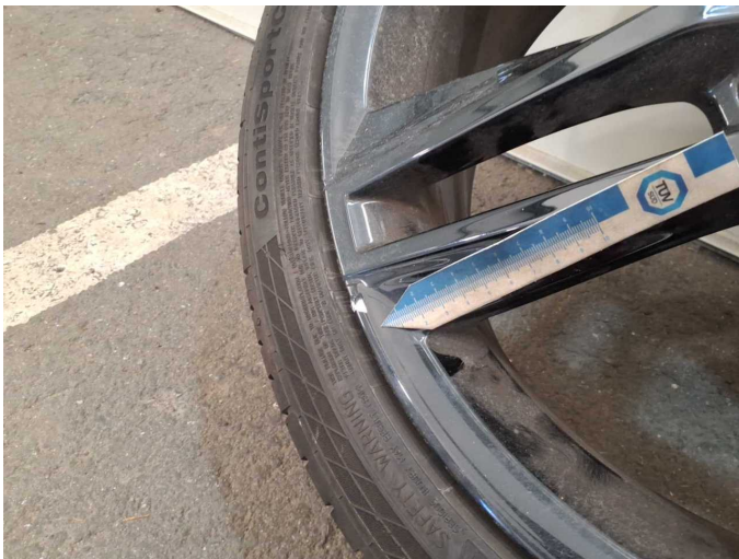
Damage 2: 2nd wheel set: 1 alloy rim - Scratch(es) - Loss in value
