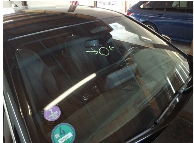
Damage #5: Vehicle glazing: Windscreen - Stone chips - Replace
