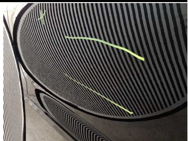
Damage #6: Door - front right side: Door - Unprofessionally repaired - Repair and paint
