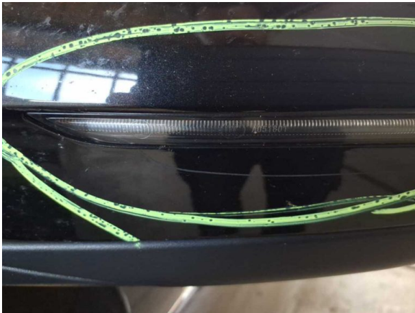
Damage #4: Wing mirror - left side: Cap - Scratched - Smart repair
