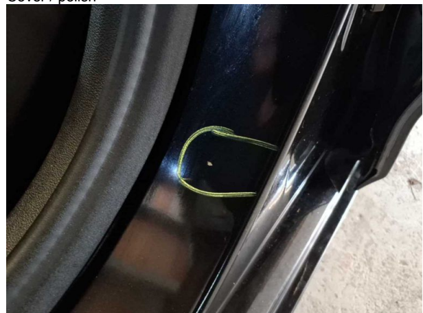
Damage #3: Sill - left side: Sill - Scratch(es) - Cover / polish
