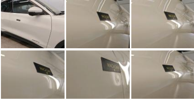
Wing RR, Bad repair, Repair and paint (complete)
