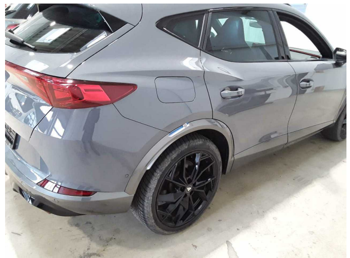
Damage 2: Side panel - rear right side: Wheel well extension - Scratch(es) - Paint
