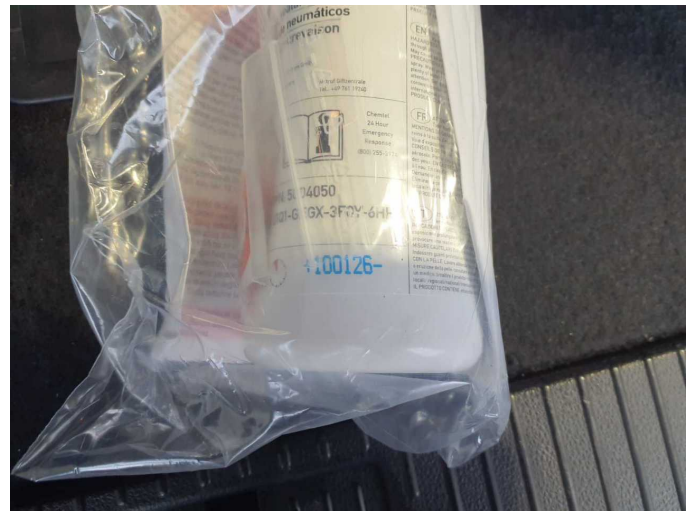
Damage 2: Equipment: Tirefit filler - Expired - Replace
