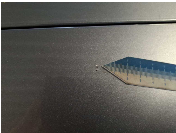
Damage 3: Bonnet: Radiator grille - Stone chips - Smart repair
