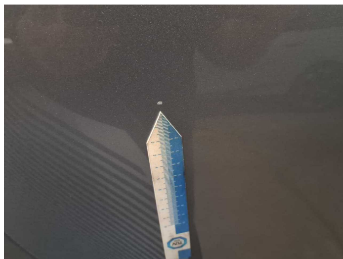
Damage 8: Side panel - rear left side: Side panel - Dent / paintcoat damage - Smart repair
