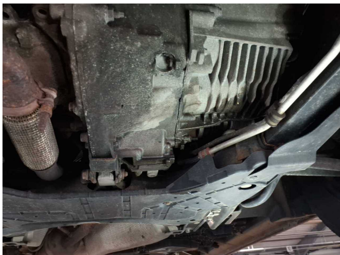
Damage 1: Gearbox: Gearbox - Leaking - Perform diagnosis
