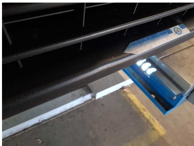
Damage 5: Front bumper: Front bumper (unpainted) - Damaged - Smart repair
