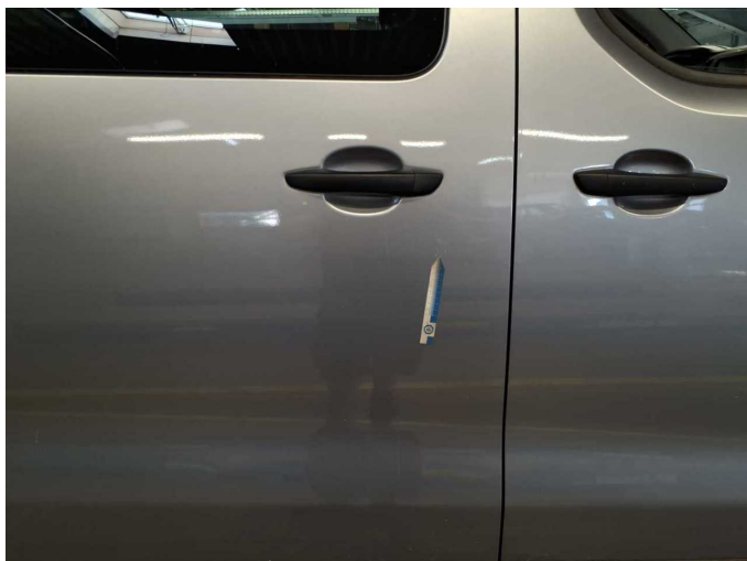
Damage 7: Sliding door, right: Sliding door - Scratched - Smart repair
