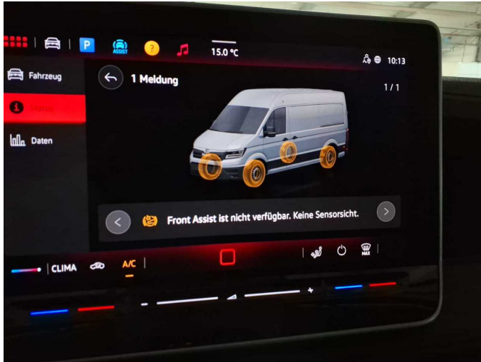
Damage 1: Instrument panel: Indicator light (Front Assist) - on - Perform diagnosis
