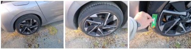
Tyre RR, Tear, Replace
