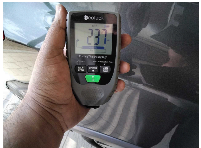
Side panel - rear right side: 237 \mu\text{m}
