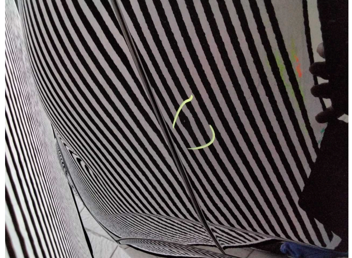
Damage 10: Side panel - rear right side: Side panel - Dent / paintcoat damage - Repair and paint
