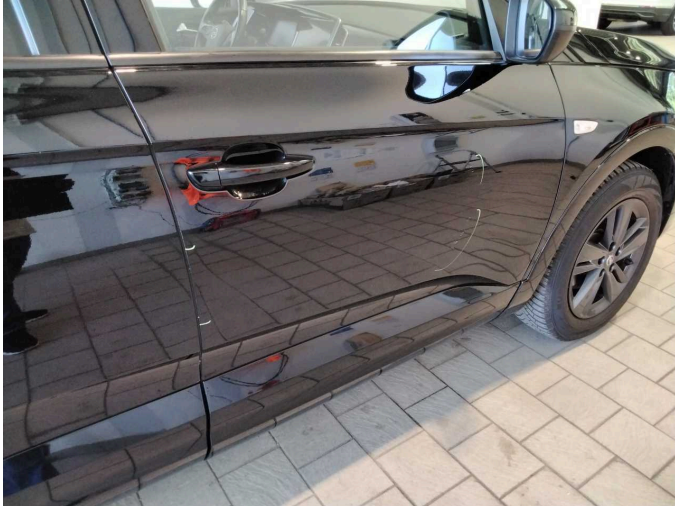
Damage 13: Door - front right side: Door - Dent / paintcoat damage - Repair and paint
