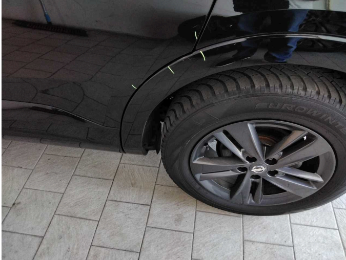
Damage 5: Side panel - rear left side: Wheel well extension - Scratch(es) - Smart repair
