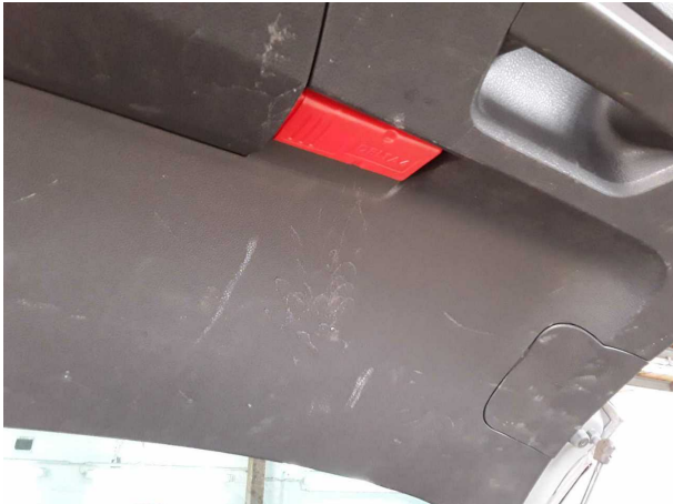
Damage #1: Trim / covers: Boot lid - interior trim - Scratched - Replace
