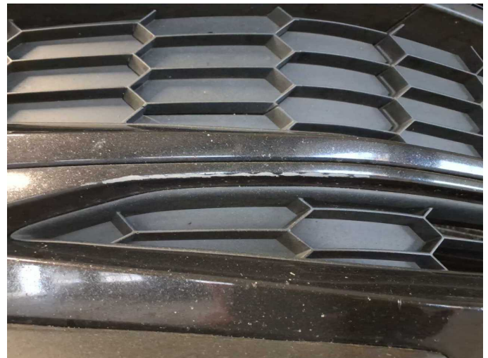
Damage 11: Front bumper: Front bumper (+verkratzt inkl. Spoiler) - Stone chips - Paint
