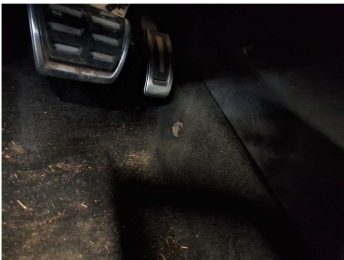
Damage 9: Trim / covers: Floor covering - front left side - Broken / torn - Smart repair
