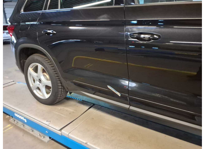
Damage 4: Door - rear right side: Door - dent(s) - Smooth repair work
