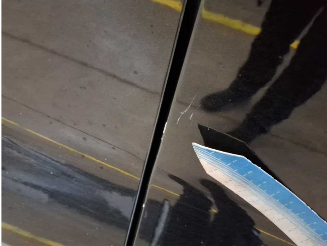
Damage 6: Door - front right side: Door - Scratch(es) - Smart repair
