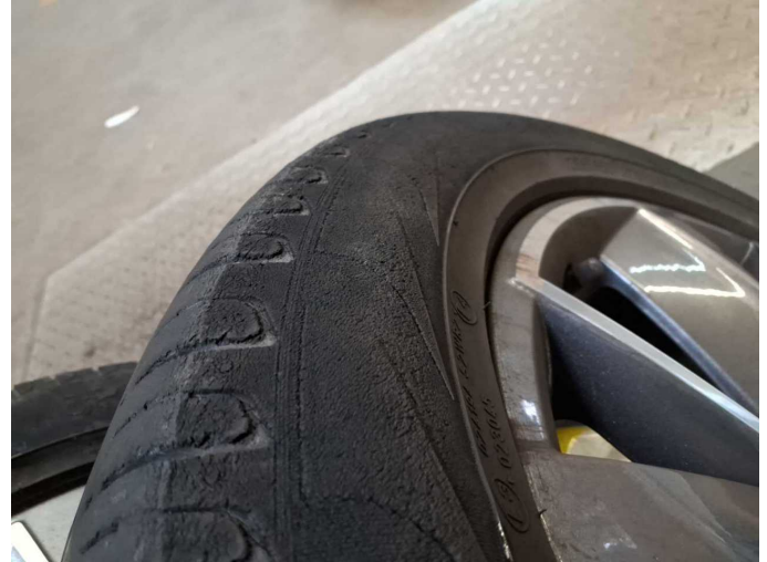
Damage 10: 2nd wheel set: 1 tyre (Flanke) - Scratched - Replace
