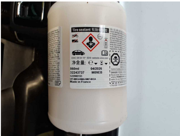
Damage #2: Equipment: Tirefit filler - Expired - Replace
