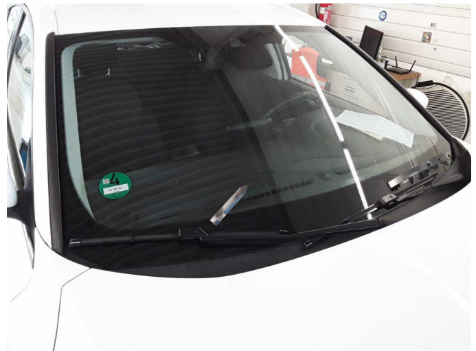
Damage 5: Vehicle glazing: Windscreen with lane departure assistant - Unprofessionally repaired - Replace
