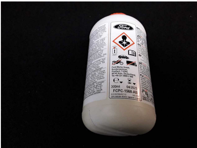
Damage 1: Equipment: Tirefit filler - Expired - Replace
