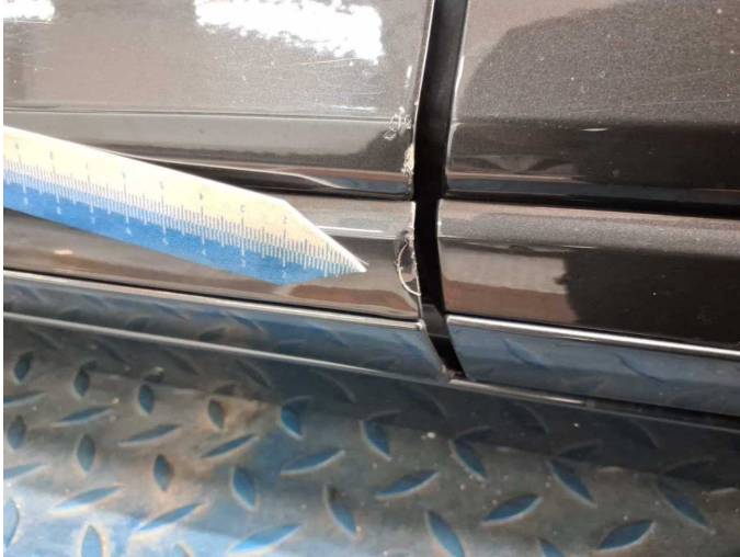
Damage 3: Door - front left side: Brightware - lower - Broken / torn - Replace
