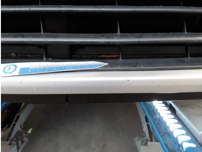
Damage 5: Front bumper: Front bumper - Scratch(es) - Paint
