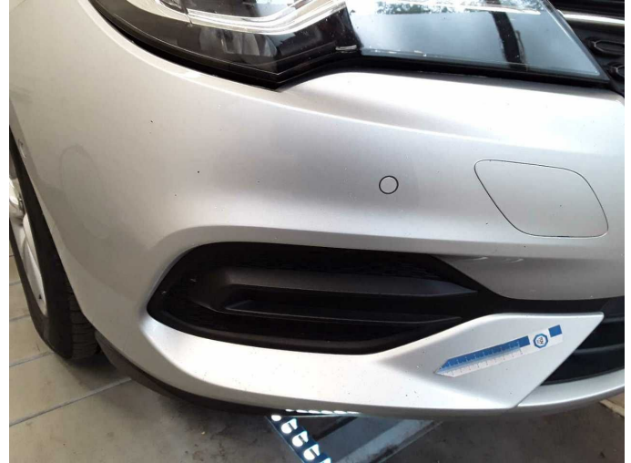
Damage 5: Front bumper: Front bumper - Scratch(es) - Paint
