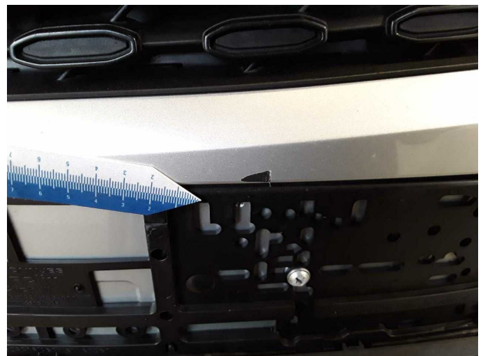
Damage 5: Front bumper: Front bumper - Scratch(es) - Paint
