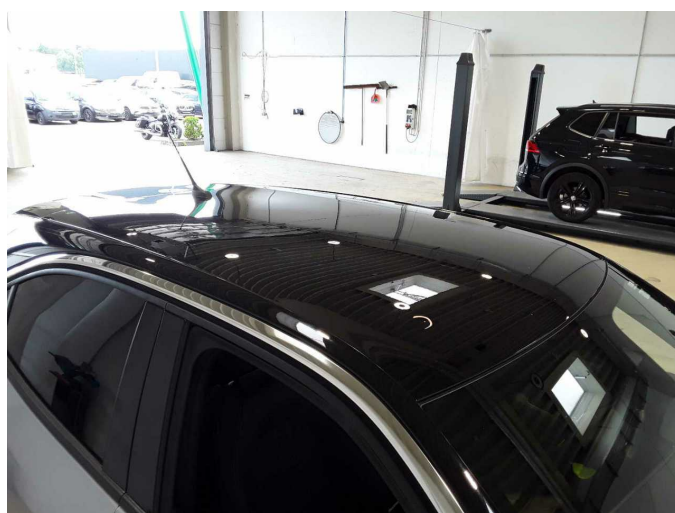
Damage 4: Roof: Roof - Damage by hail - Repair
