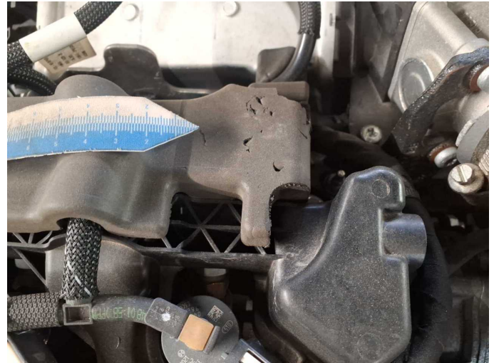
Damage 1: Misc.: Misc. (Isolierug Motor) - Damage caused by marten / rodent - Replace
