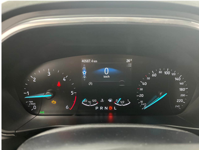
Damage 4: Instrument panel: Indicator light (Motorkontrolle aktiv) - on - Perform diagnosis
