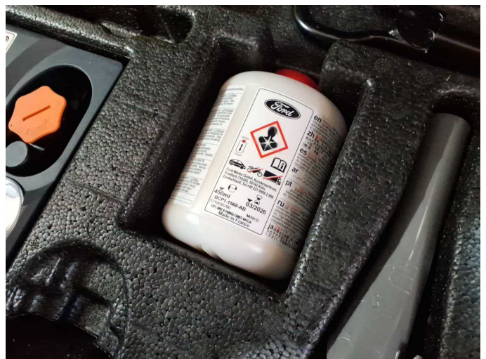
Damage 3: Equipment: Tirefit filler - Expired - Replace
