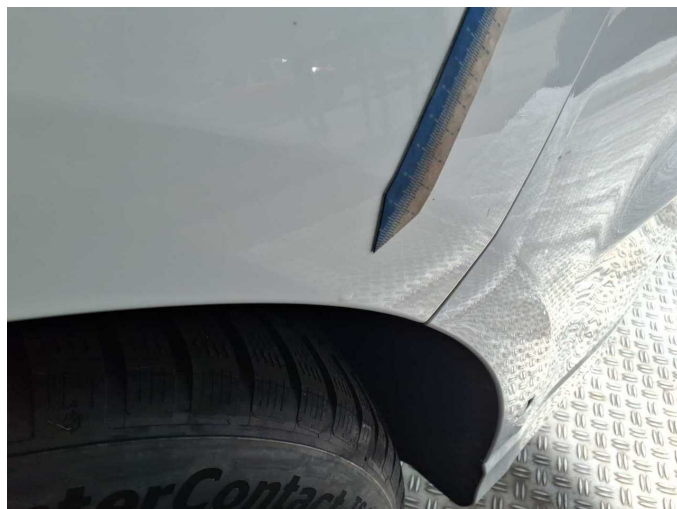
Damage 10: Side panel - rear left side: Side panel - Corrosion - Smart repair
