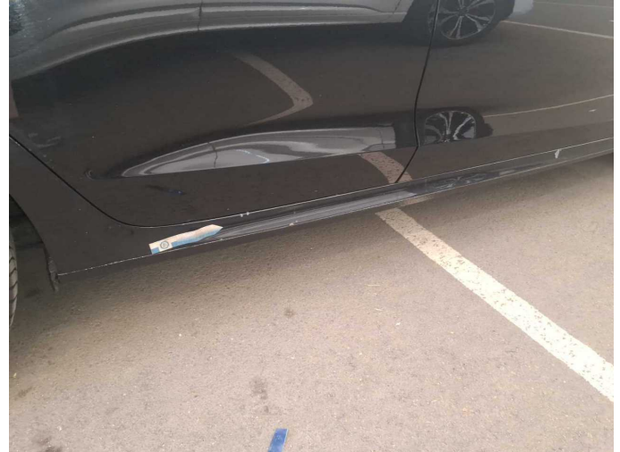
Damage 3: Sill - right side: Sill - Paint defect - Repair and paint
