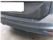
Bumper R, Scratch(es), Repair and paint (complete)
