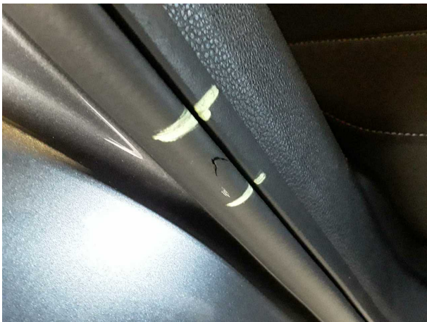
Damage #2: Door - rear right side: Door seal - Damaged - Replace
