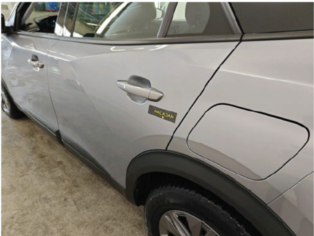
Door RL Scratch(es) Repair and paint (complete) Left
