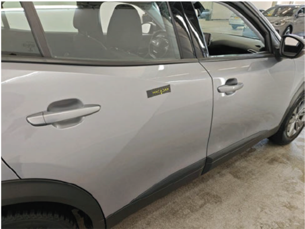
Door RR Bad repair Repair and paint (complete) Right
