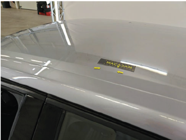
Roof Dent(s) Repair and paint (complete) Roof & others
