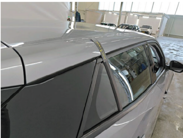
Roof pillar R Chemical polution Repair and paint (complete) Right
