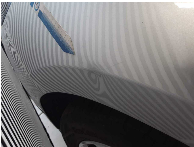
Damage 9: Mudguard - left side: Mudguard - left side - Dent / paintcoat damage - Repair and paint
