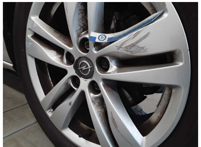
Damage 5: Wheel / tyres: Alloy rim - front right side - Scratched - Smart repair
