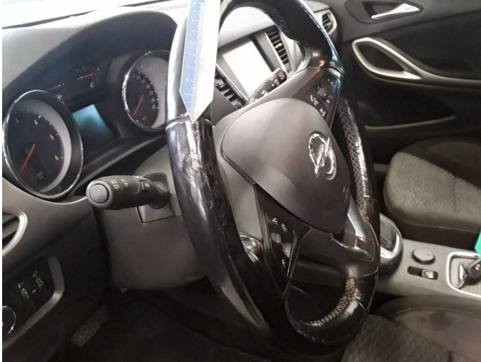
Damage 3: Steering system: Steering wheel - Worn - Smart repair
