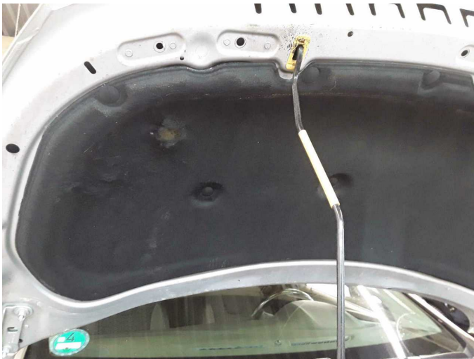
Damage 7: Bonnet: Insulation lining - Damaged - Replace
