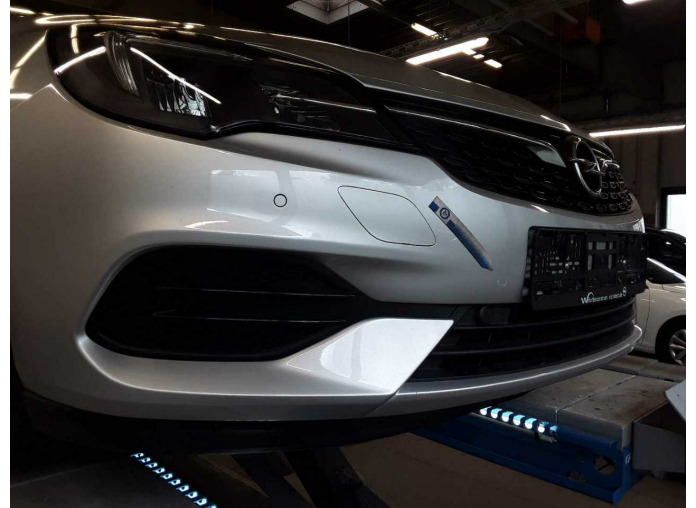
Damage 4: Front bumper: Front bumper - Scratch(es) - Smart repair
