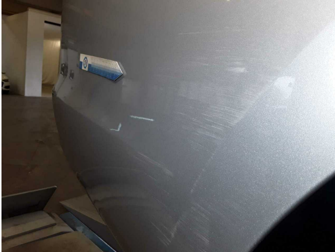
Damage 8: Rear bumper: Rear bumper - Scratched - Paint
