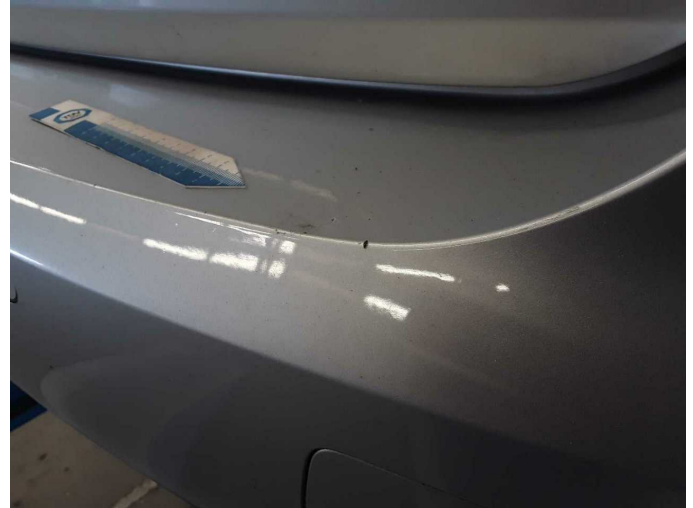
Damage 8: Rear bumper: Rear bumper - Scratched - Paint
