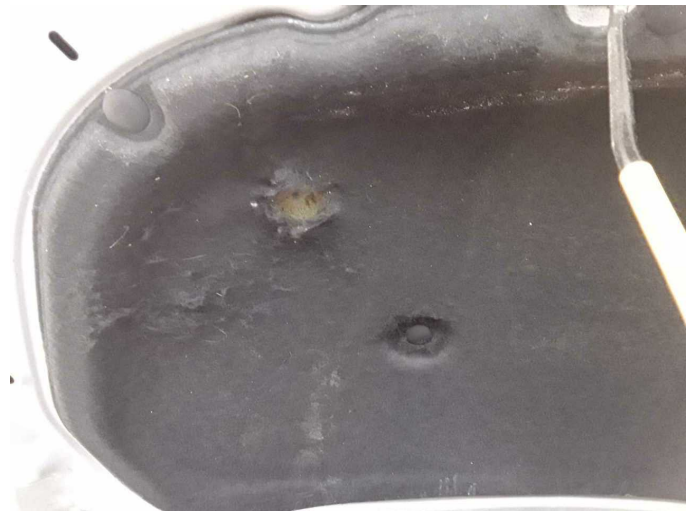
Damage 7: Bonnet: Insulation lining - Damaged - Replace
