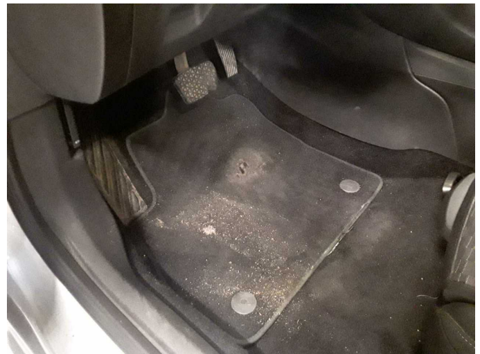
Wear and tear 6: Trim / covers: Floor mats - Damaged - No deduction
