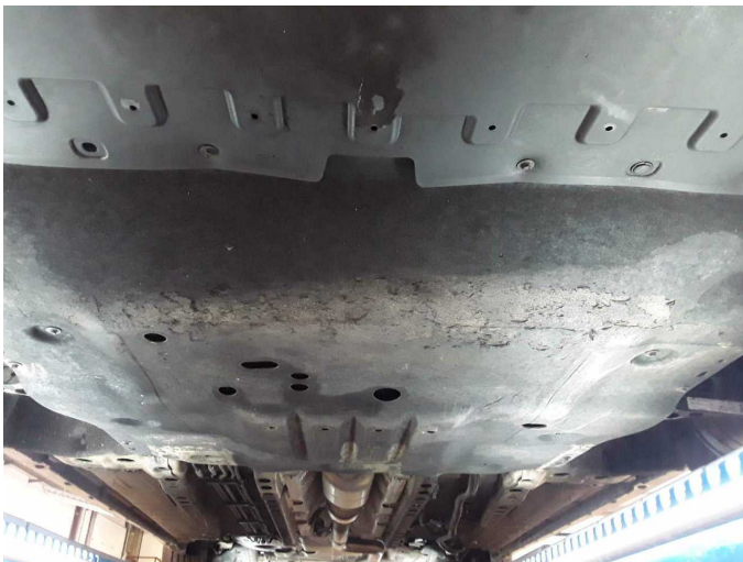
Wear and tear 2: Body: Underbody panelling - Scratched - No deduction
