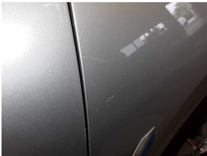
Damage 11: Side panel - rear left side: Side panel - Dent / paintcoat damage - Repair and paint
