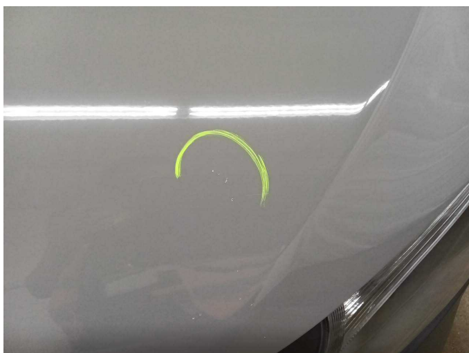
Damage 4: Bonnet: Bonnet - Stone chips - Paint
