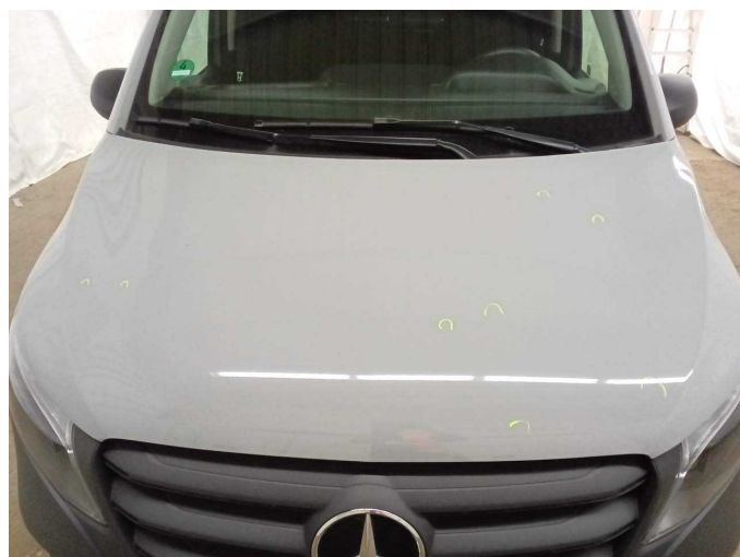
Damage 4: Bonnet: Bonnet - Stone chips - Paint
