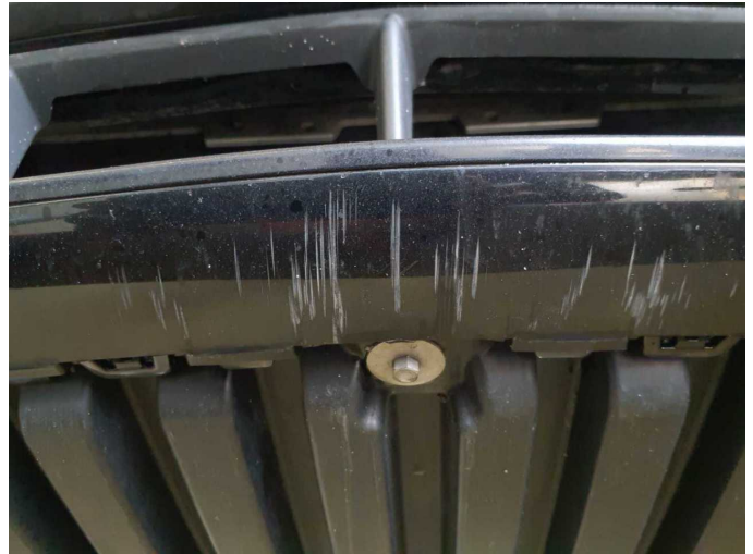
Damage 9: Front bumper: Front bumper - Scratch(es) - Paint
