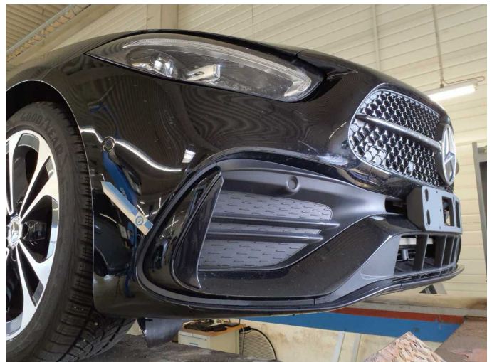
Damage 9: Front bumper: Front bumper - Scratch(es) - Paint
