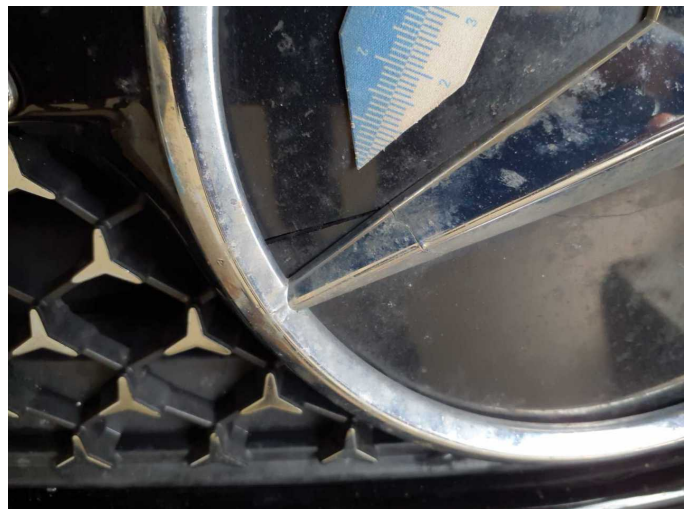
Damage 1: Front structure: Emblem - Broken / torn - Replace
