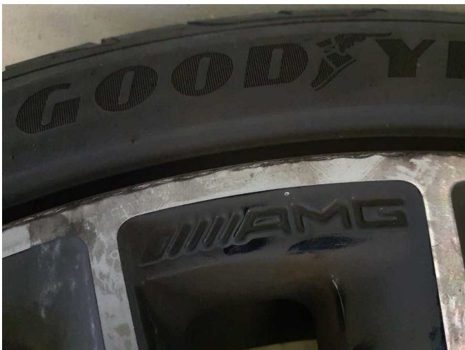
Damage 8: 2nd wheel set: 1 alloy rim - Scratched - Replace
