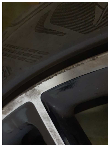
Damage 8: 2nd wheel set: 1 alloy rim - Scratched - Replace
