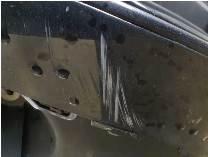
Damage 9: Front bumper: Front bumper - Scratch(es) - Paint
