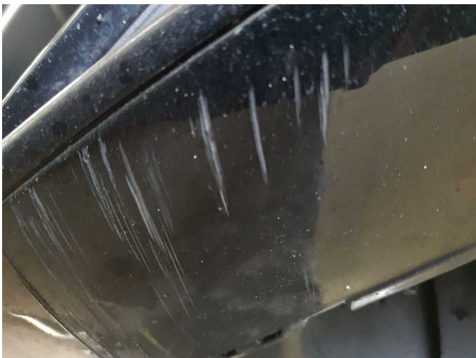
Damage 9: Front bumper: Front bumper - Scratch(es) - Paint
