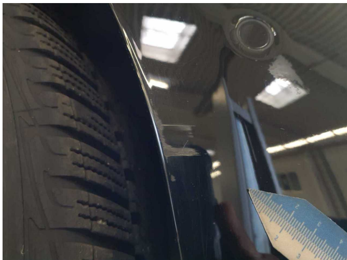
Damage 9: Front bumper: Front bumper - Scratch(es) - Paint
