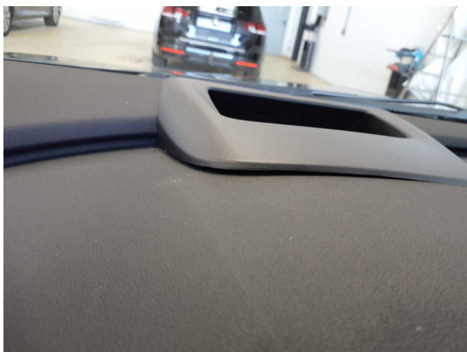
Damage 1: Trim / covers: Trim / covers - Malposition - Repair
