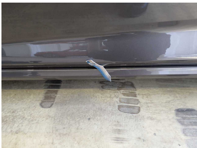
Damage 6: Sill - left side: Trim - Scratch(es) - Smart repair
