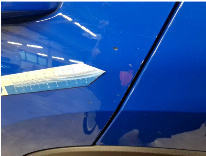
Damage 3: Door - rear left side: Door - Scratched - Paint
