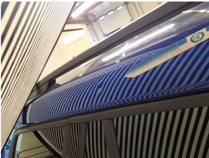
Wear and tear 3: Roof: Roof rail - right side - dent(s) - No deduction
