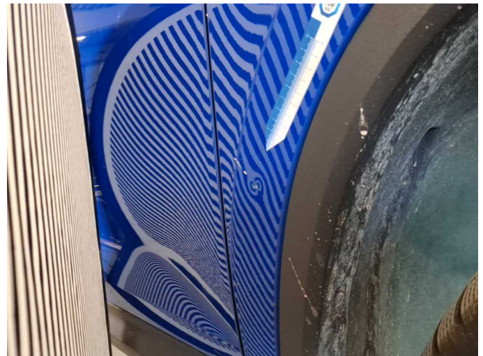
Damage 2: Mudguard - right side: Mudguard - right side - Dent / paintcoat damage - Smart repair
