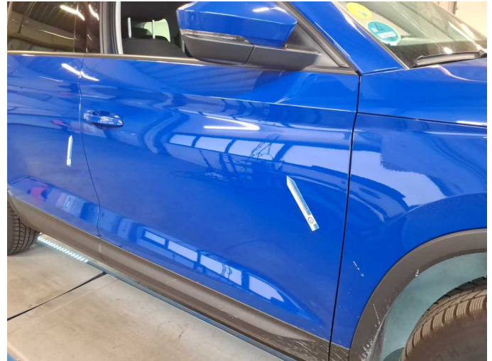
Damage 5: Door - front right side: Door - Dent / paintcoat damage - Paint
