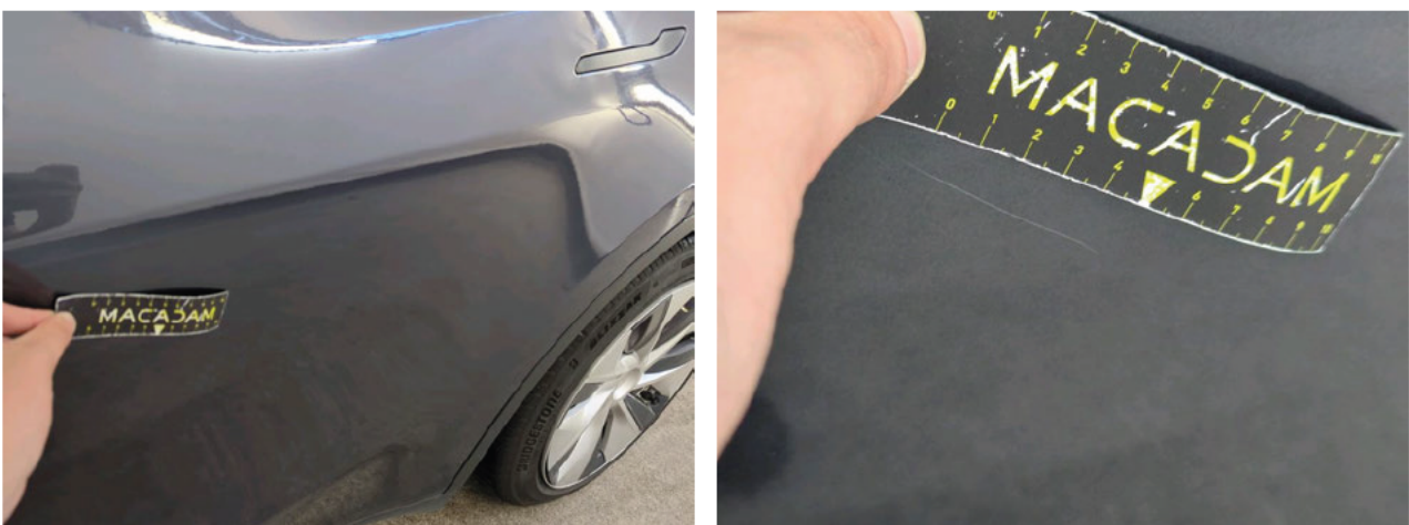
Door RL Scratch(es) Repair and paint (complete) Left
