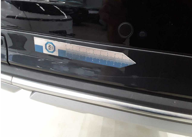
Damage 4: Rear bumper: Rear bumper (Incl. Blende grau) - Scratched - Repair and paint
