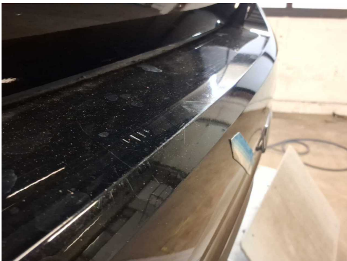
Damage 11: Rear bumper: Rear bumper - Scratched - Paint
