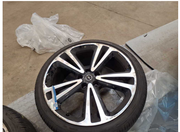
Damage 13: 2nd wheel set: 3 alloy rims (Materialabtrag) - Scratched - repair according to calculation
