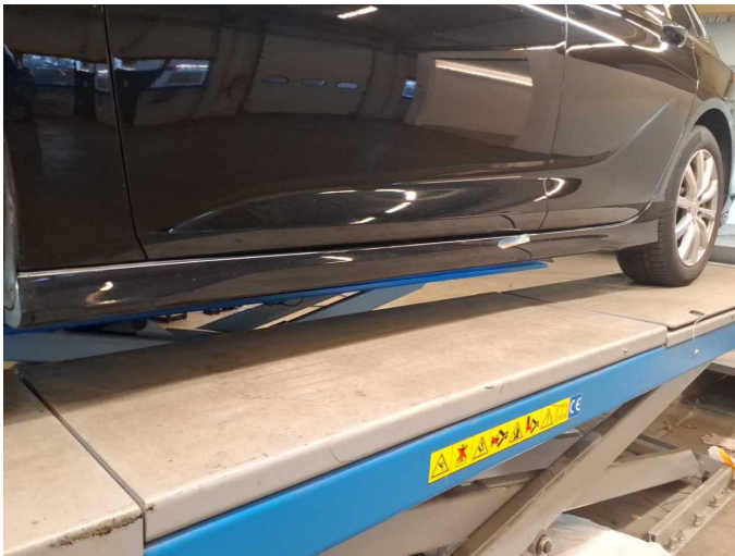
Damage 5: Sill - left side: Trim - Scratched - Smart repair
