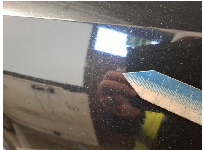
Damage 12: Front bumper: Front bumper - Stone chips - Paint
