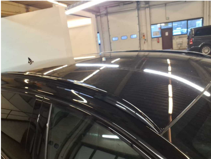
Damage 2: Roof: Roof - dent(s) - Smooth repair work
