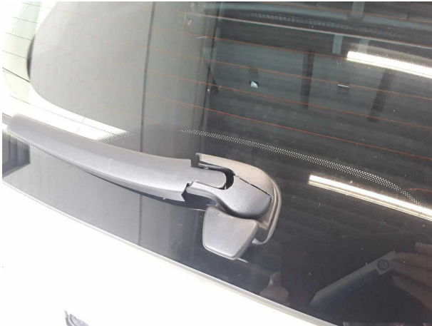
Damage #1: Screen cleaning: Wiper arm - rear (Deckel) - Broken / torn - Replace
