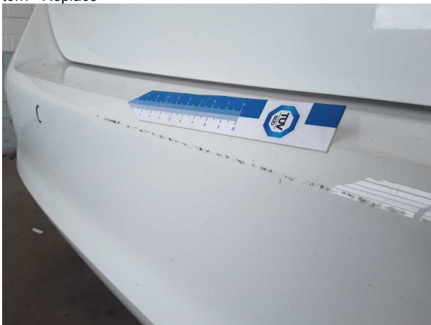
Damage #2: Rear bumper: Rear bumper - Scratched - Paint
