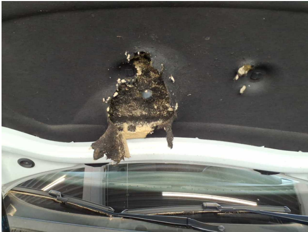
Damage #1: Bonnet: Insulation lining - Holes - Replace
