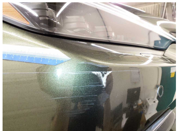
Damage 2: Front bumper: Bumper with Parktronic - Scratched - Smart repair
