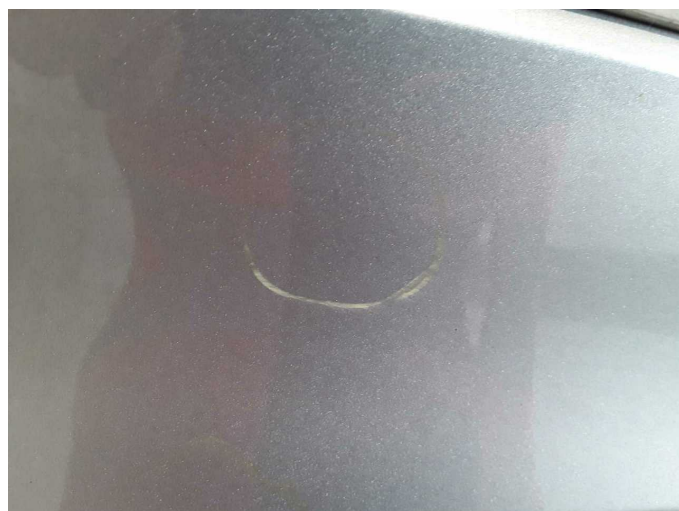
Damage 2: Door - front right side: Brightware - lower - Scratch(es) - Paint
