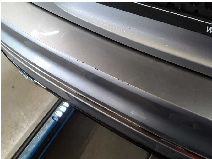
Damage 3: Rear bumper: Rear bumper - Scratched - Paint
