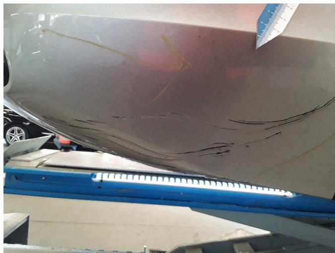
Damage 3: Rear bumper: Rear bumper - Scratched - Paint
