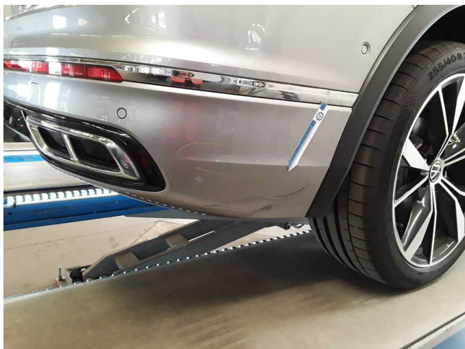
Damage 3: Rear bumper: Rear bumper - Scratched - Paint
