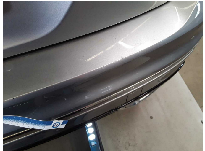
Damage 3: Rear bumper: Rear bumper - Scratched - Paint
