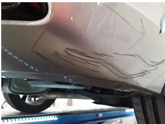
Damage 3: Rear bumper: Rear bumper - Scratched - Paint
