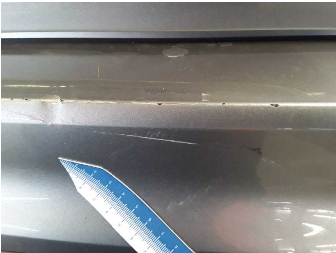
Damage 3: Rear bumper: Rear bumper - Scratched - Paint
