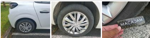
Tyre RL, Out of tolerance, Replace
