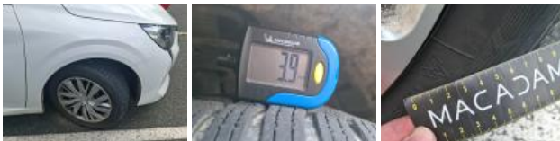
Tyre RR, Out of tolerance, Replace
