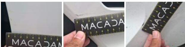
Rear bulkhead lining, Scratch(es), Smart repair
