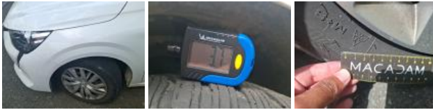
Tyre FR, Out of tolerance, Replace
