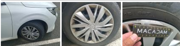
Wheel cover FR, Deformed / Strained, Replace
