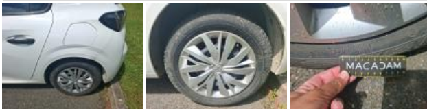
Wheel cover FR, Deformed / Strained, Replace
