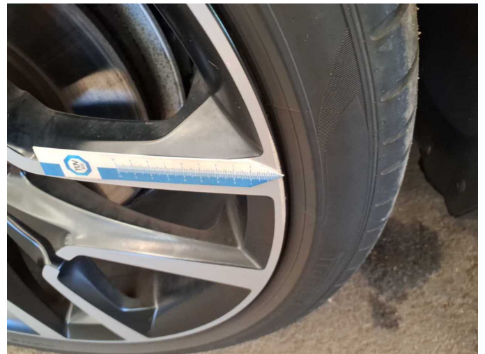
Damage 5: Wheel / tyres: Alloy rim - front left side - Scratch(es) - Loss in value
