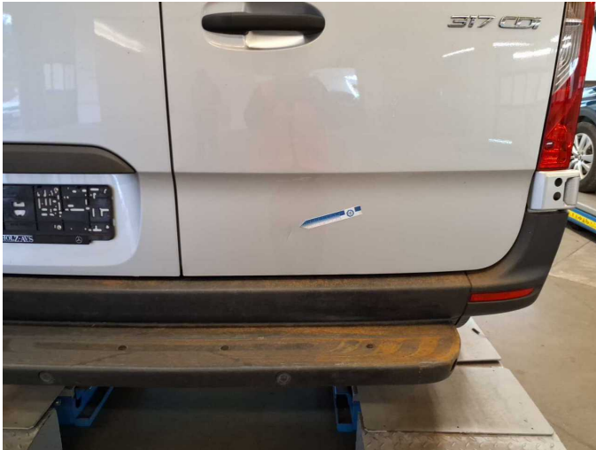
Damage 5: Boot lid / rear door: Rear door - right side - Dent / paintcoat damage - Repair and paint
