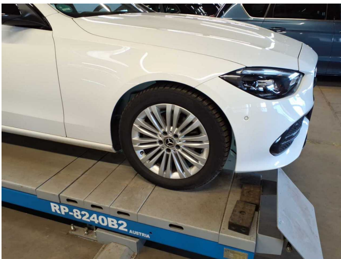
Damage 4: Wheel / tyres: Alloy rim - front right side - Scratch(es) - Loss in value
