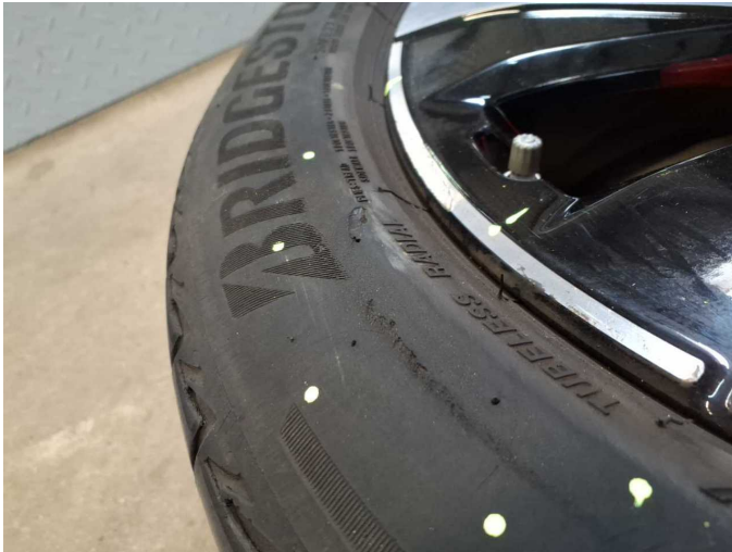
Damage 3: 2nd wheel set: 1 tyre (Flanke) - Damaged - Replace
