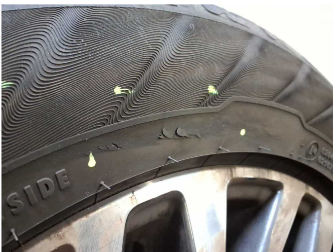
Damage 5: 2nd wheel set: 1 tyre (Flanke) - Damaged - Replace
