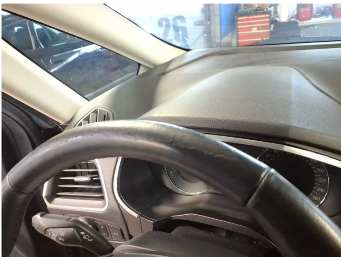
Damage 2: Steering system: Steering wheel - Abrasion - Smart repair
