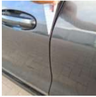
Damage Type Door-edge chipped
