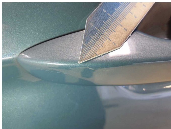
Wear and tear 6: Door - rear left side: Door handle - outside - Scratch(es) - Smart repair
