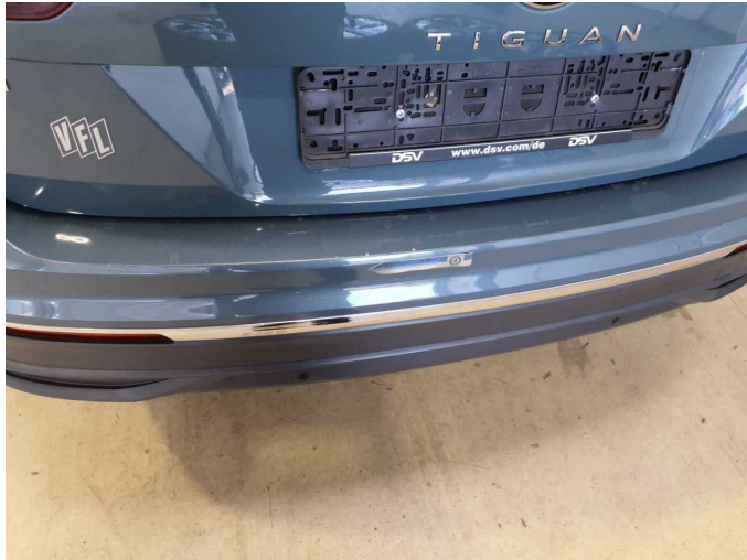
Damage 14: Rear bumper: Rear bumper - Scratch(es) - Paint
