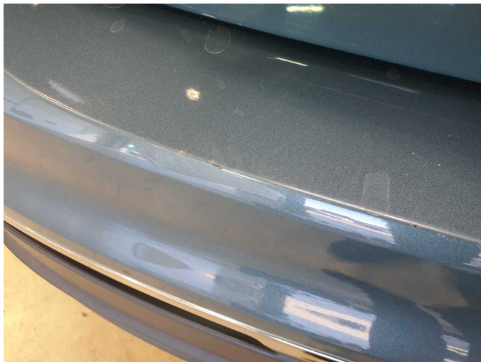
Damage 14: Rear bumper: Rear bumper - Scratch(es) - Paint
