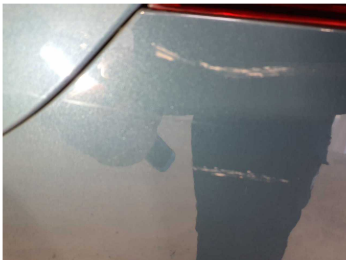
Damage 14: Rear bumper: Rear bumper - Scratch(es) - Paint
