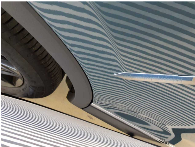
Damage 8: Door - rear right side: Door (Einschlüsse und Spachtel rissig) - dent(s) - Smart repair
