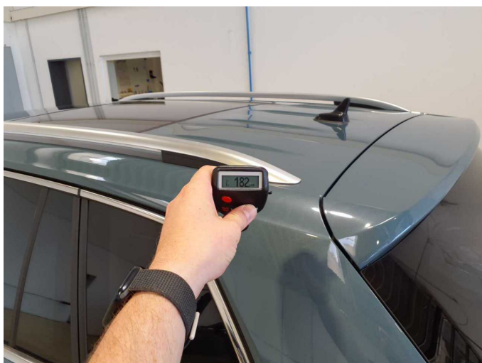
Repainting 1: Roof rail - left side
