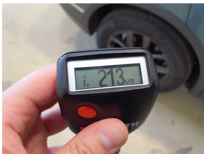
Repainting 3: Side panel - rear right side
