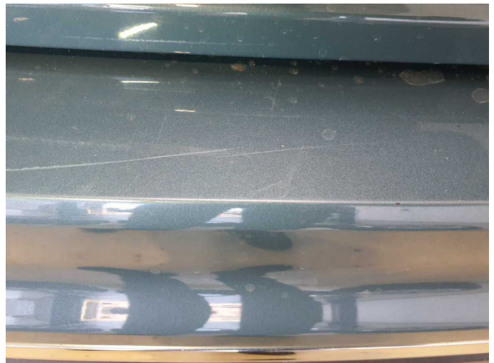
Damage 14: Rear bumper: Rear bumper - Scratch(es) - Paint
