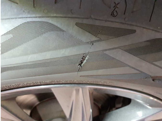
Damage 7: Wheel / tyres: Tyre - rear right side (nicht fahrbereit) - Broken / torn - Replace
