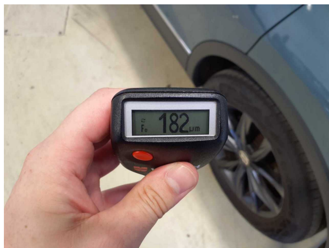
Repainting 1: Roof rail - left side
