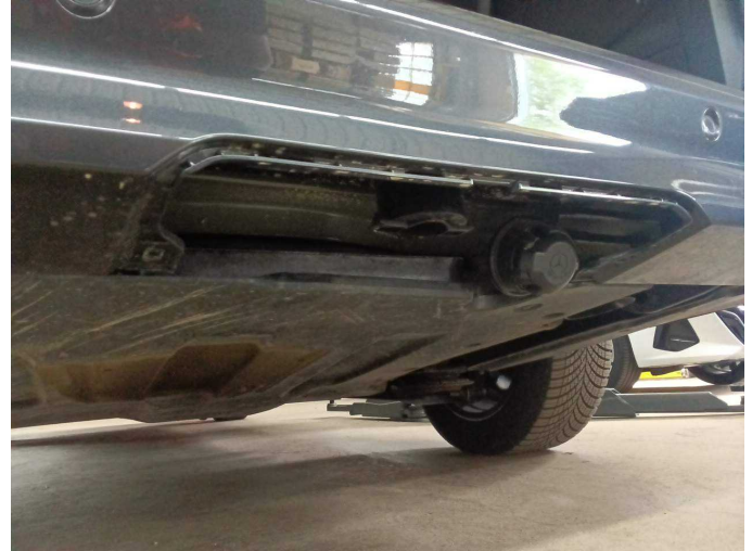
Damage 6: Rear of vehicle: Trailer hitch (Anhängerabdeckung fehlt) - Missing - Perform
