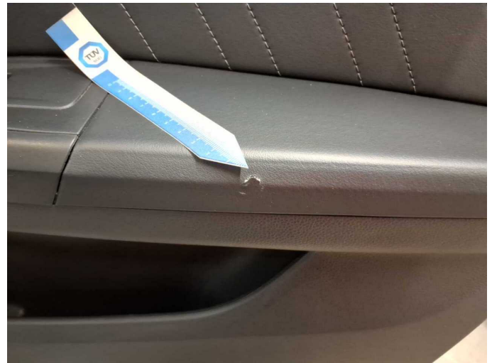
Damage 2: Trim / covers: Door trim - front left side - Holes - Smart repair
