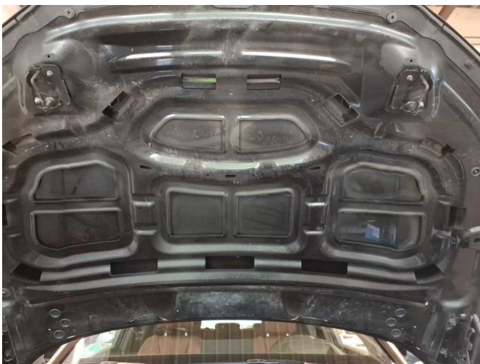
Damage 2: Bonnet: Insulation lining - Missing - Replace
