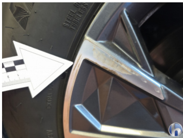
9. Felge Hinten - Links Kratzer - Smart Repair
