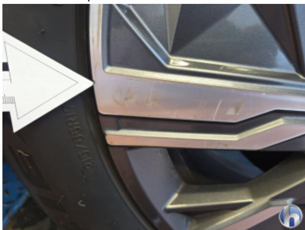
9. Felge Hinten - Links Kratzer - Smart Repair
