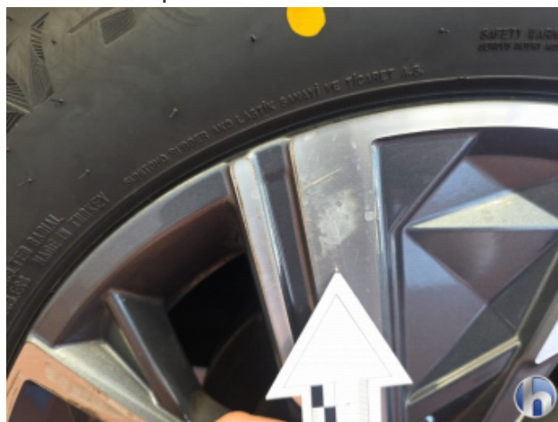
9. Felge Hinten - Links Kratzer - Smart Repair
