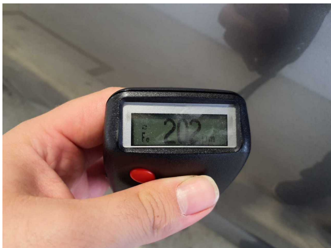
Repainting 1: Door - front left side
