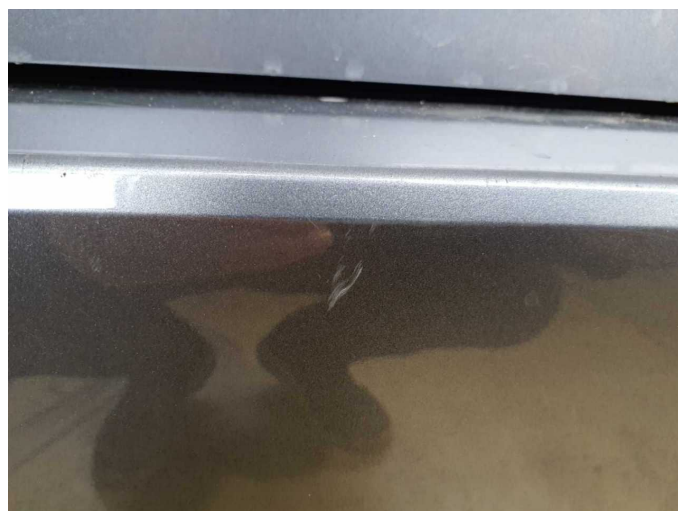
Damage 4: Rear bumper: Rear bumper - Scratch(es) - Paint
