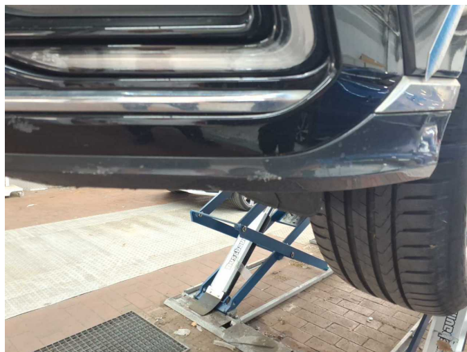
Damage 6: Front bumper: Front bumper - Scratch(es) - Paint
