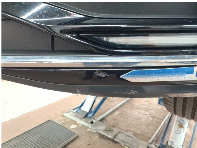
Damage 4: Front bumper: Cover bumper - front - Scratch(es) - Replace
