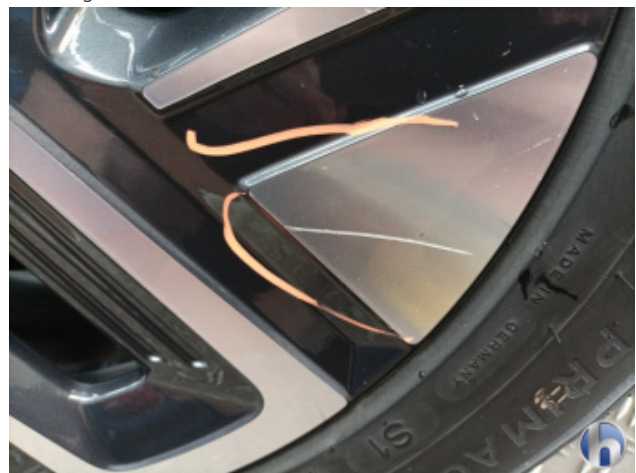
1. Felge Hinten - Links Kratzer - Smart Repair
