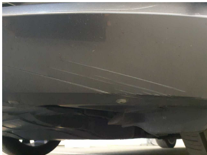
Damage 11: Front bumper: Front bumper - Scratch(es) - Repair and paint
