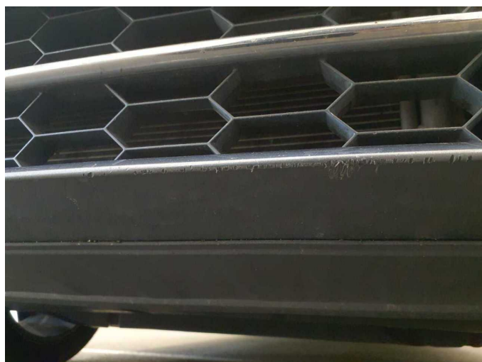
Damage 11: Front bumper: Front bumper - Scratch(es) - Repair and paint
