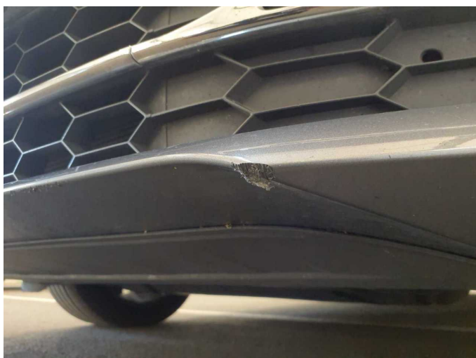
Damage 11: Front bumper: Front bumper - Scratch(es) - Repair and paint
